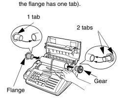
**6** Pull the empty spool toward the back of the compartment, unwinding the film as you pull.
